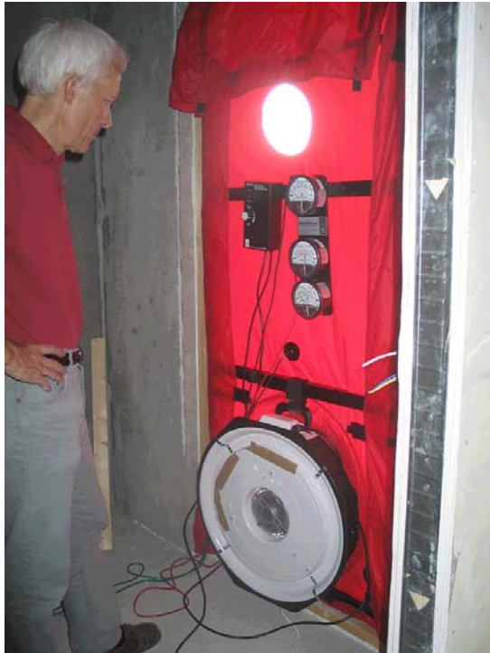
Fig. 1. Blowerdoor test in apartment.
