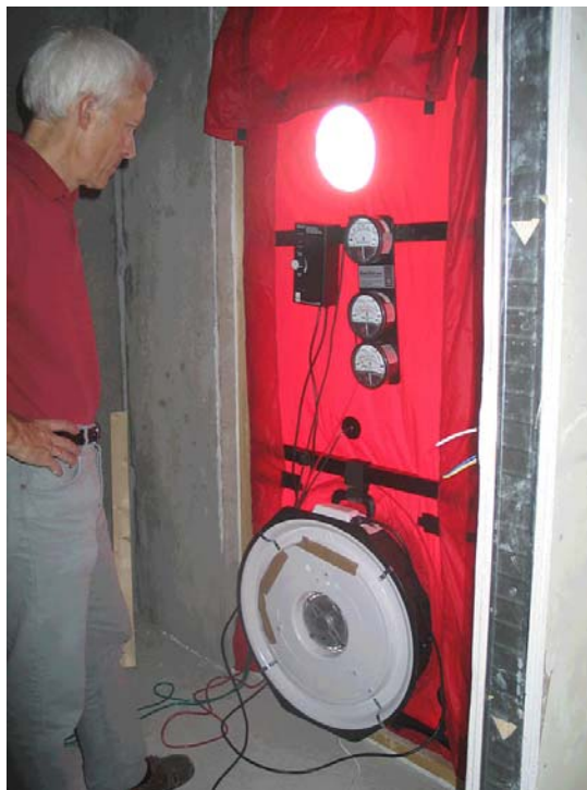
Fig. 1. Blowerdoor test in apartment.
